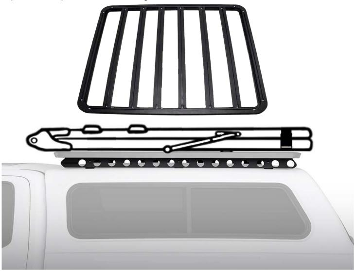
ENSURE TENT IS CLOSED AND OVER THE CENTRE LATCHES ARE FULLY SECURED DURING FITMENT
