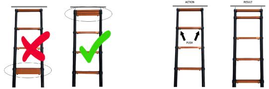
If further shortening is required press the second set of locking buttons (third rung from the top). This will close the 85mm gap until rung 1 & 2 are now touching. Swing in the bottom of the ladder until it supports the weight of the roof top tent. If the angle of the ladder is between  $70^{\circ}$  and  $75^{\circ}$ , this adjustment is complete.
