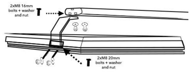
**Note:** The roof bars supplied with the Saber Super Fly roof top tent are not designed to carry significant loads. A maximum of 10kg can be carried on top of the Saber Super Fly providing this weight is spread evenly amongst the two bars Load weights greater than 20kg will void any warranty.
