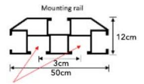
Slide mounting bolt in to either channel.
