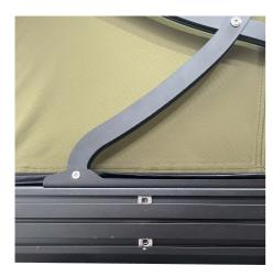
1. Slide in two of the channel nuts, one in the top channel, one in the lower in desired awning bracket position.
