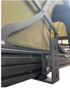
2. Allign your bracket with the channel nuts and insert the washer first, then the M8 bolts in line with the nuts
