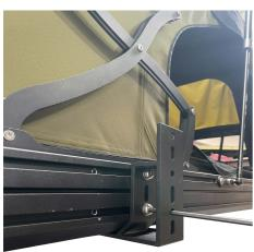
3. Using a 5mm Allen key tighten the nuts, you can use the existing holes in the brackets to make the process easier.
