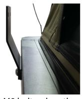
3. Using 2 M8 bolts, place the raised window fly plate into the channel nuts ensuring the backing plate is attached on inside.
