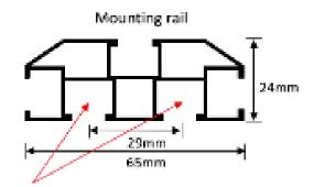
Slide mounting bolt in to either channel.
