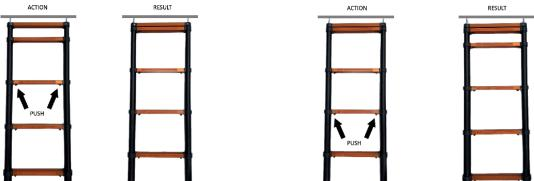
**NOTE:** When height adjusted, the ladder will only lock in the downward position. If further adjustment is required, repeat the above steps by continuing the sequence by depressing the next set of locking buttons.
