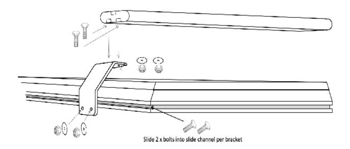
**Note:** The roof bars supplied with the Saber roof top tent are not designed to carry significant loads. A maximum of 20kg can be carried on top of the Saber providing this weight is spread evenly amongst all three bars. Load weights greater than 20kg will void any warranty. When adding additional weight to the top of the Saber consideration must be given to the overall weight rating capacity of your vehicle's roof and roof rack.
