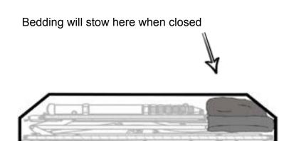
**NOTE:** The amount of bedding left in tent may affect closure. If tent is not folding and closing smoothly, bedding may be too bulky and must be removed. Forcing closure may put undue pressure on components and cause failure which will not be covered by warranty.
