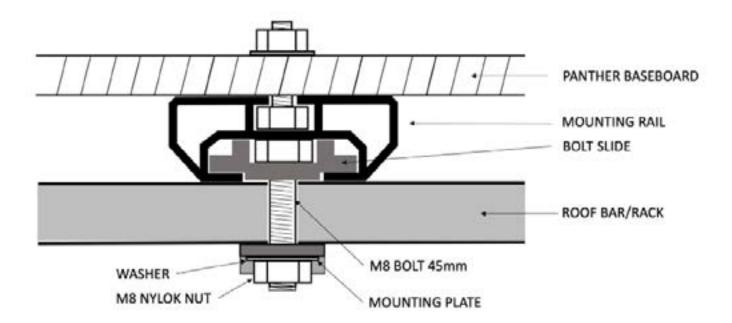
Inspect the position of the roof top tent to ensure it will open in the desired position. Place a mounting plate under the roof bar whilst locating the bolts and hand tighten Nylok nut. Repeat for all 4 corners. Double check the tent's position as desired and tighten all nuts securely with 13mm spanner. Insert end caps into the ends of the mounting rails, this may require light taps with a hammer
