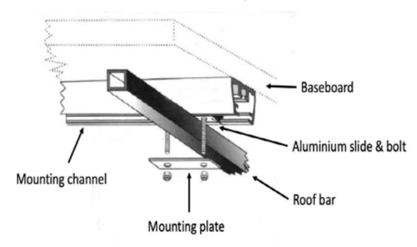
Inspect the position of the roof top tent to ensure it will open in the desired position. Place a mounting plate under the roof bar whilst locating the bolts and hand tighten Nylok nut. Repeat for all 4 corners. Double check the tent's position as desired and tighten all nuts securely with 13mm spanner. Insert end caps into the ends of the mounting rails, this may require light taps with a hammer.
