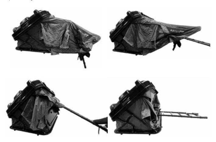
5. Retract ladder and secure with hook & loop strap.
